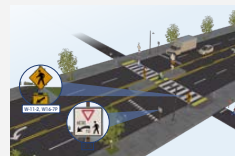
Rectangular Rapid Flashing Beacon (RRFB) Source: Federal Highway Administration
